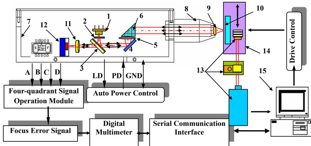
Fig.6 Schematic of grating pitch measurement. (10 grating plate, other components are the same as Figure 4)
