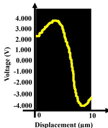
Fig.4 Calibrated FES S-curve
