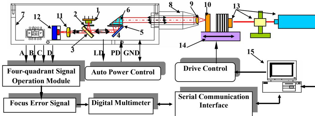
Fig.5 The setup of measuring FES curve. ( 1 laser diode, 2 grating, 3 polarized beam splitter&1/4 wave plate, 4 reflector, 5 collimation lens, 6 transition reflector, 7 probe case, 8 head case, 9 holographic Fresnel lens, 10 optical reflector, 11 cylindrical lens, 12 four-quadrant photodiode, 13 laser interferometer, 14 precision stage, 15 PC)
